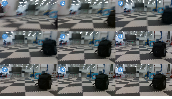
Fig. 3: Image blurring phenomenon. This figure shows the occurrence of image blurring in the robot view, which impacts the clarity and accuracy of the processed images.
