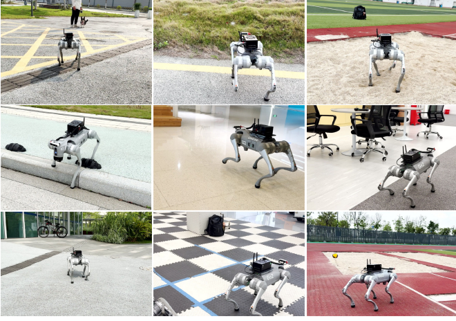
Fig. 6: Environment adaptation. LOVON excels in open-world object navigation, effectively adapting to a wide range of objects and environments.
